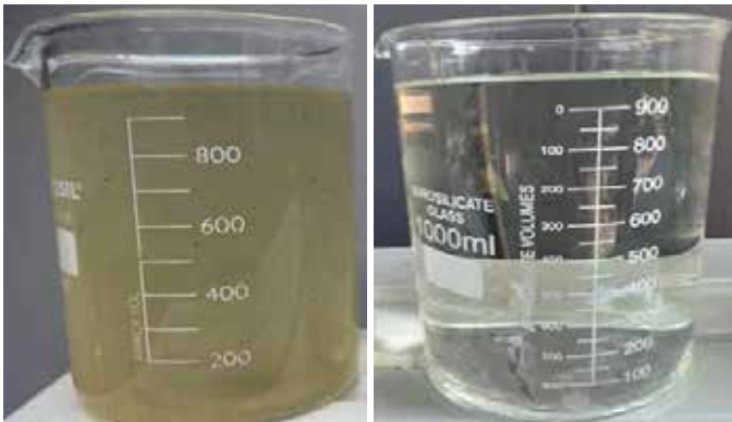
Sewage Sample Treated at the TADOX Plant Before & After
