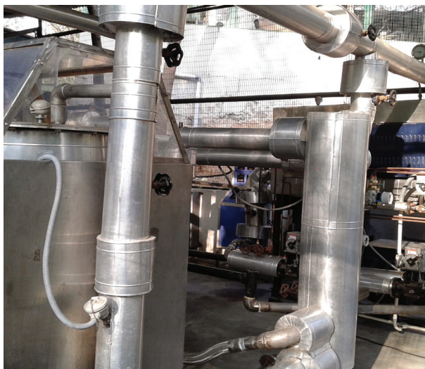
TERI's patented gas-fired auger continuous pilot pyrolysis unit (20 kg/h max)
