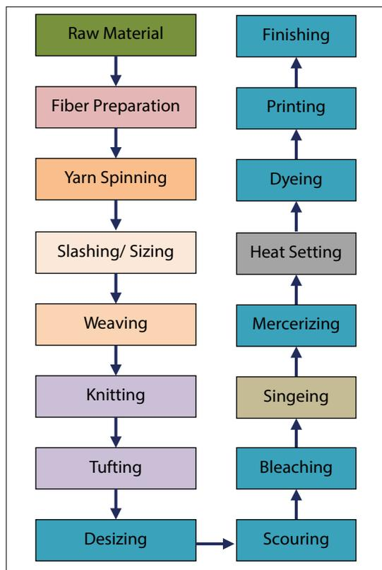
Figure 4 Processes & water usage areas in a textiles industry
