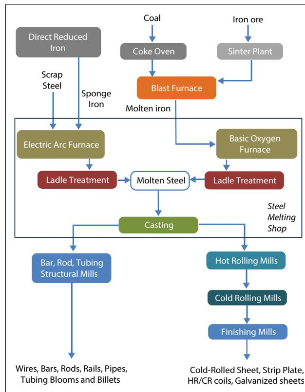
Figure 5 Processes & water usage areas in an iron & steel industry
