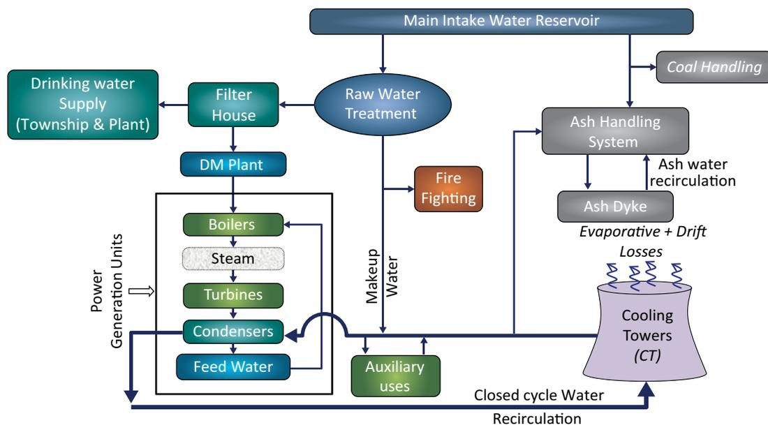
**Figure 2** Processes & water usage areas in a thermal power plant
