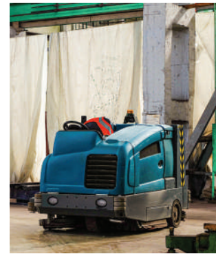
(4) Track out- Paving of track at construction site and clean-up of track out through road sweeper or wet broom or manual sweeping
