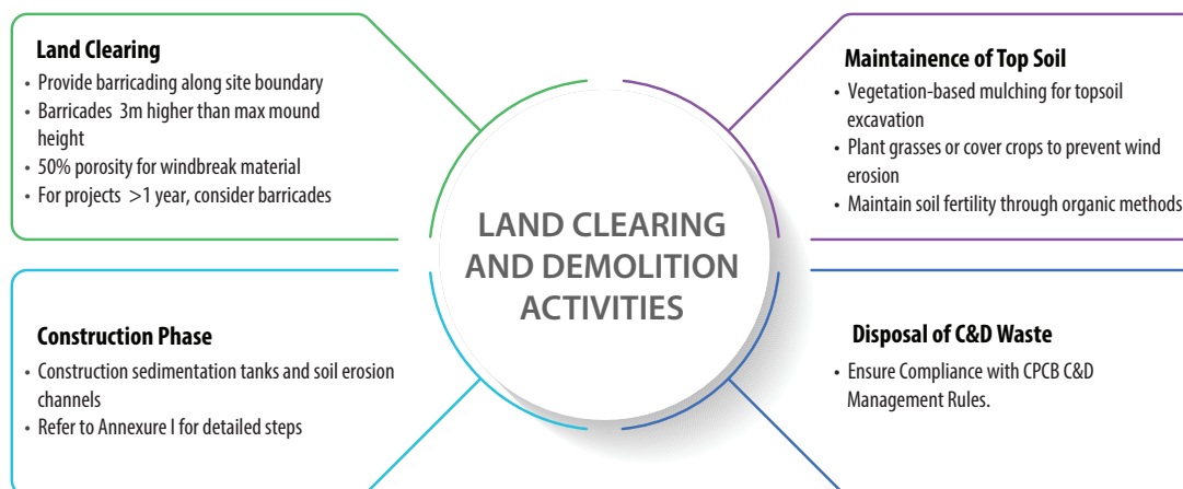
Land Clearing and Demolition Activities
