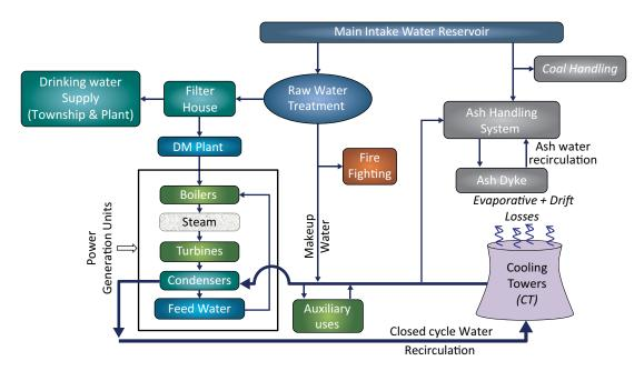
Figure 2 Processes & water usage areas in a thermal power plant
