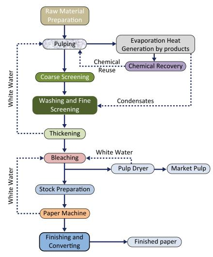
Figure 3 Processes & water usage areas in a pulp & paper industry
