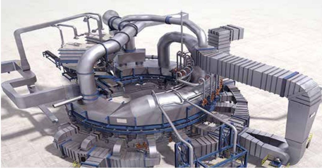
Figure 19: 3D view of Circular Pelletization Technology
