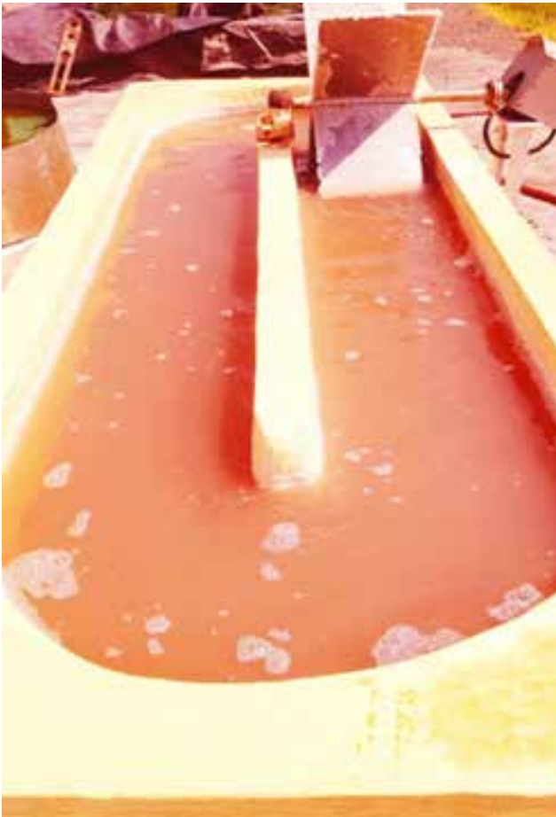
▶ Beta-carotene producing algal cultivation in the Mumbai coast using 1000 litres raceway pond (the alga has changed colour from green to orange when beta-carotene production shift happened)
