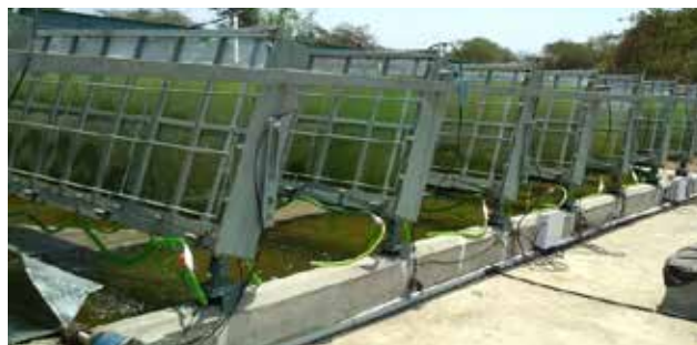
► Marine algal cultivation in 100,000 litres (220 sq. m) production system (based on sunlight distribution and 6000 litres raceway pond inoculum system) for improvement and production of 3rd generation feedstock (to use as platform feed for biodiesel, bioethanol, biohydrogen, aquafeed, and animal feed) production.
