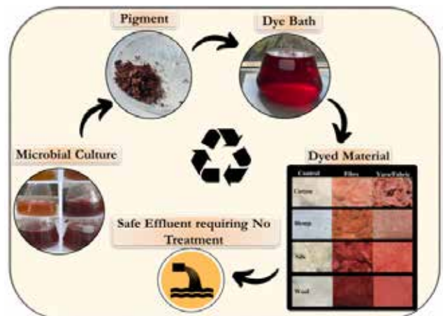
► In-house developed microbial dye production and textile dyeing process with cellulosic and proteinaceous fibres along with safe effluent discharge without any chemical treatment
