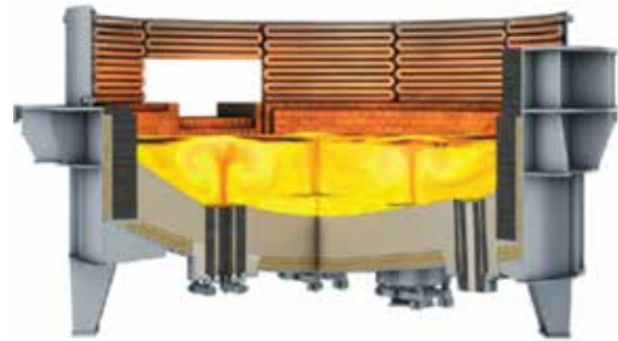
Figure 19: Inert gas stirring system
