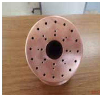
Photograph showing cross section of a high efficiency oxy-fuel burner
