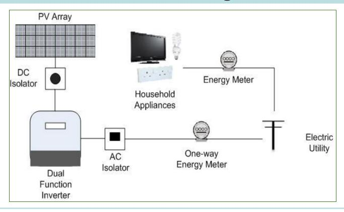
It is a simple and cost effective Rooftop Solar PV system which doesn't affect household grid connection and wiring.
