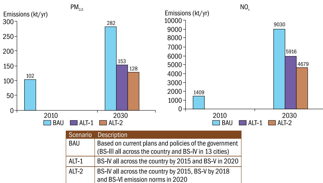
**Figure 5:** PM and NO<sub>x</sub> emission reduction in 2030 in vehicular sector due to introduction of BS-VI norms in 2020.
